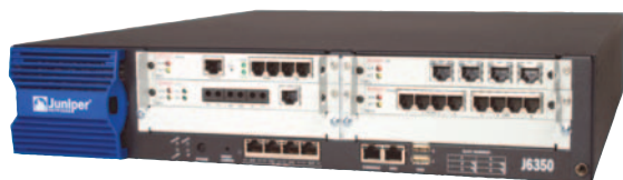
Avaya IG550 Gateway in Juniper J6350 Router
